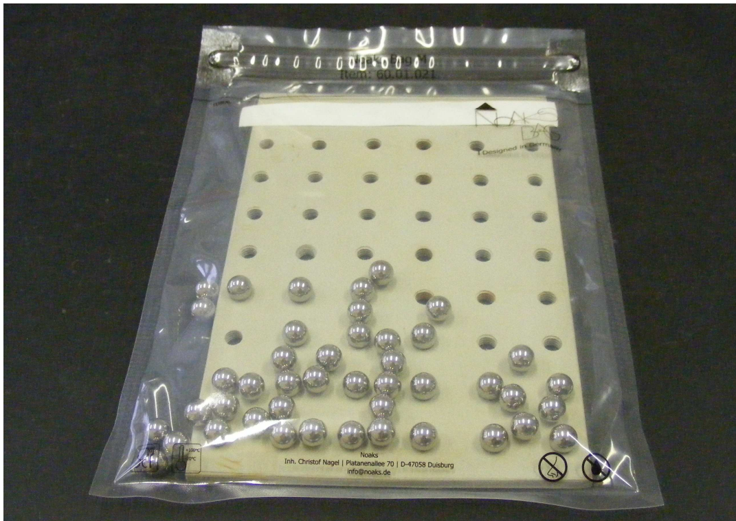
figure 2 specimen No. 5 after IP Code X8 Test, exemplary
